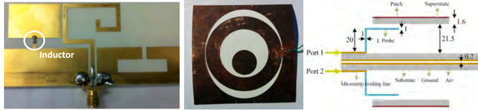
Fig. 3. Multi-band UHF RFEH antennas: Triple band antenna with a lumped inductor and three radiator elements [21] (left), triple band slotted patch [16] (center), and L-probe-fed dual-band patch [22] (right)
